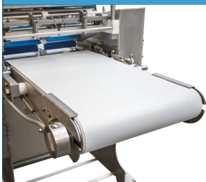
Short outfeed conveyor ≈-549mm
